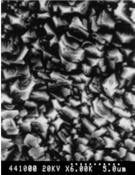
Fig. 4. SEM micrograph for Zn–Ni alloy deposit with 15.34% nickel content.
