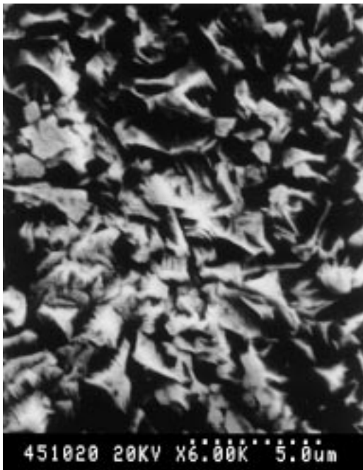
Fig. 5. SEM micrograph for Zn–Ni alloy deposit with 17.25% nickel content.
